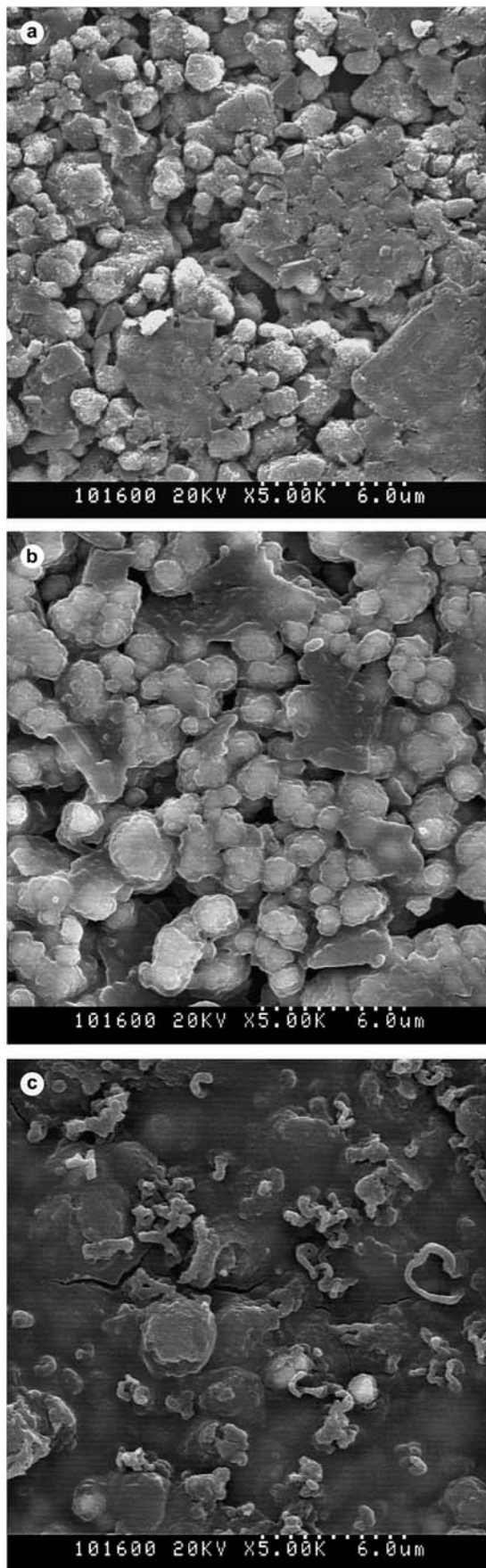
Fig. 4. SEM images of the \text{LiCoO}_2 electrode taken from the overcharged cells containing: (a) no additives, (b) 5 wt % xylene, at the beginning of overcharge and (c) 5 wt % xylene, at 100% overcharge.
